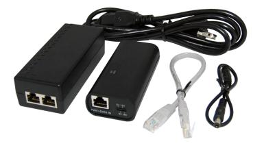
Alfa APOE591218V is an PoE set with adjustable output power 5V, 9V, 12V,18V; a revolutionary technology for powering Ethernet terminals such as IP Telephone sets, wireless access point, and Internet protocol camera. The technology incorporates electrical power into a LAN data line enabling the delivery of operating power in addition to data communicate to terminals over standard cabling infrastructure.
