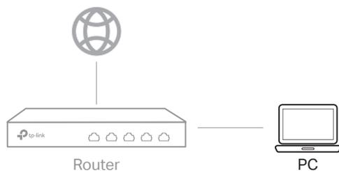
1. Connect a computer to a LAN port of the router with an RJ45 cable properly. If your computer is configured with a fixed IP, change it to **Obtain an IP address automatically**.
