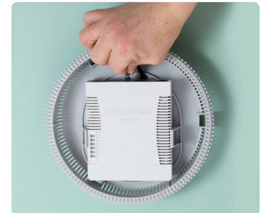
13 Connect all cables and close the Cover.
