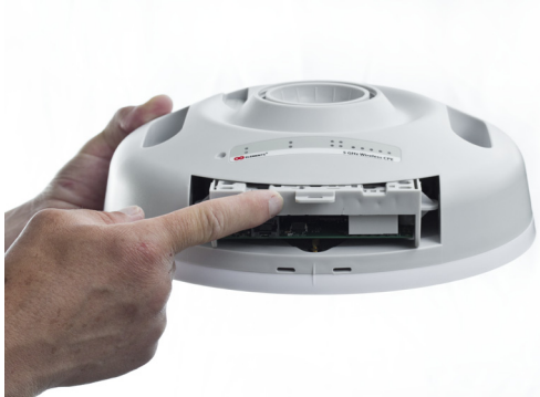
4 Insert the Chassis into the StationBox. Insert pigtails first, then slide the Chassis.
