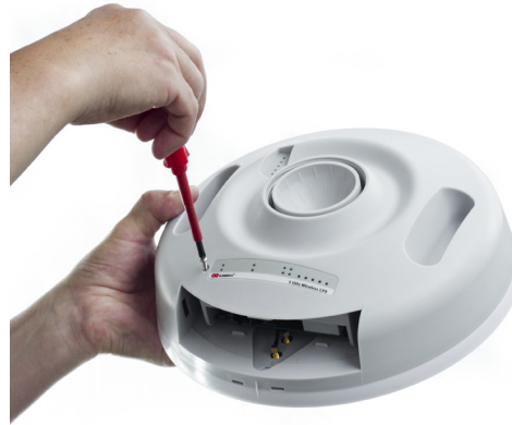
5 Use the Security Screw to secure the Chassis (optional).
