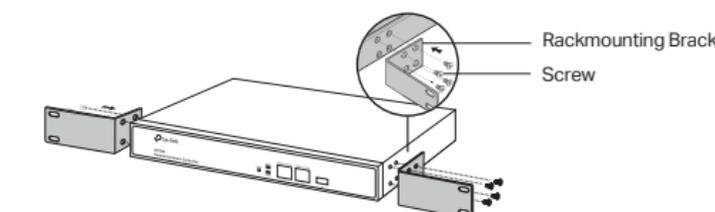
3. After the brackets are attached to the device, use suitable screws (not provided) to secure the brackets to the rack.
