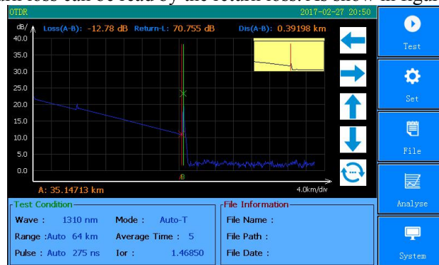
Fig.3-6 Reflection loss test
