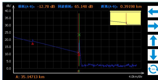
Fig.3-10 Return loss measurement
