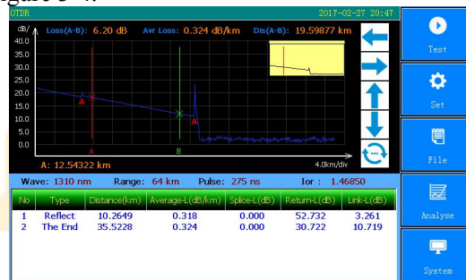
Fig.3-4 Average Loss Test
