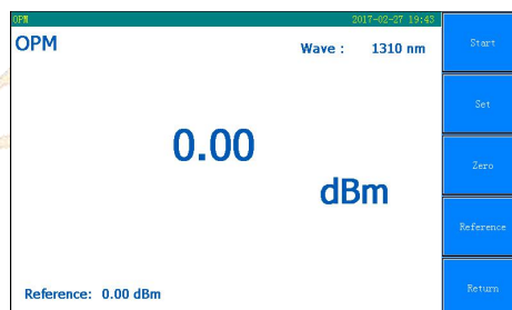
Fig.4-1 Optical power meter test interface
