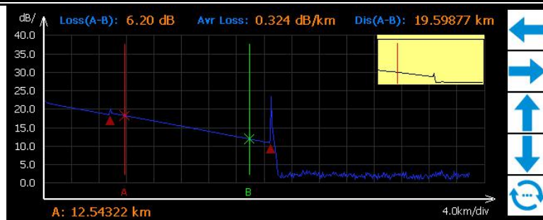
Fig.3-8 Average Loss Measurement
