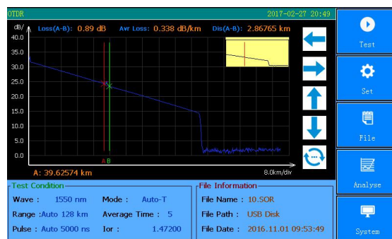
Fig.3-5 Connection Loss Test
