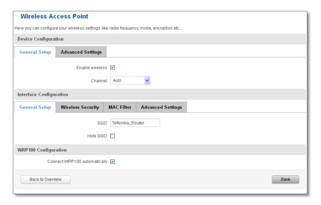
Here you can see the Overview of the wireless configuration. It is divided into two main sections – device and interface. One is dedicated to configuring hardware parameters other – software.
