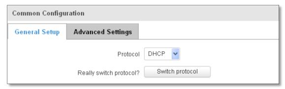
You can switch between the Static, DHCP or PPPoE protocol by selecting the protocol that you want to use and then pressing **Switch Protocol**.
