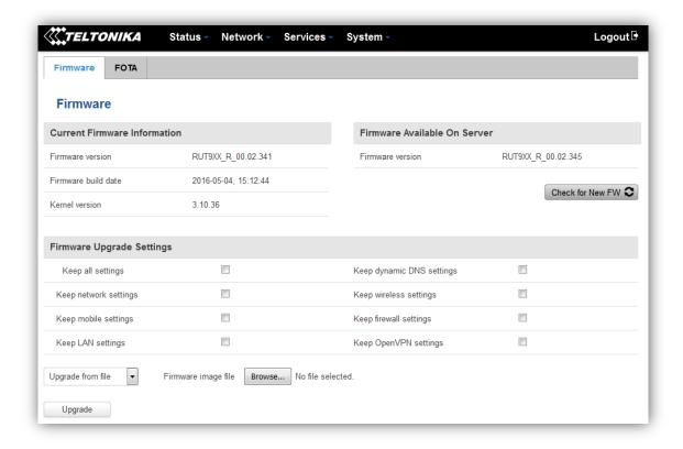
**Keep all settings** – if the check box is selected router will keep saved user configuration settings after firmware upgrade. When check box is not selected all router settings will be restored to factory defaults after firmware upgrade. When upgrading firmware, you can choose settings that you wish to keep after the upgrade. This function is useful when firmware is being upgraded via Internet (remotely) and you must not lose connection to the router afterwards.
