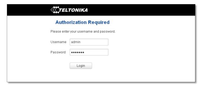
Enter the default password, which is "admin01" into the "Password" field and then either click Login with your mouse or press the Enter key. You have now successfully logged into the RUT900!
