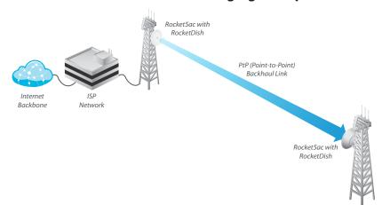
The Rocket R5AC-Lite radios paired with the RocketDish RD-5G31-AC antennas create a powerful PtP backhaul link.
