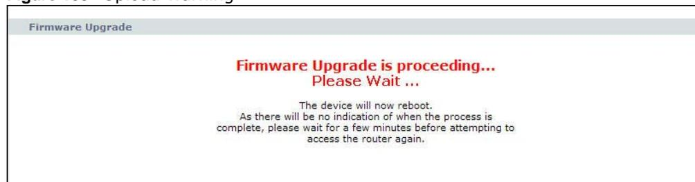
The NBG-418N v2 automatically restarts in this time causing a temporary network disconnect. In some operating systems, you may see the following icon on your desktop.
