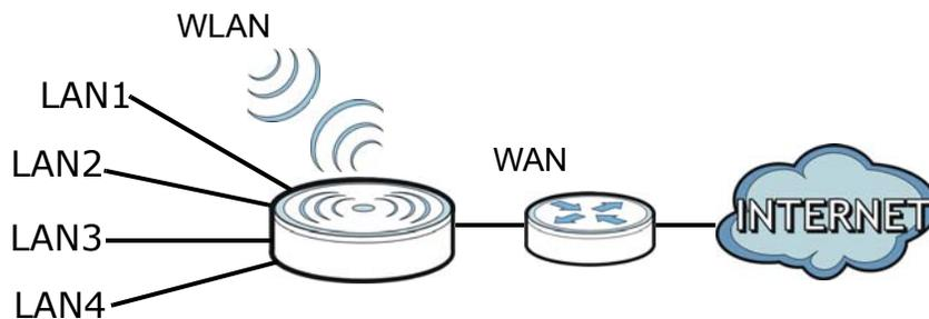
You can set up the NBG-418N v2 with other IEEE 802.11b/g/n compatible devices in one of the following device modes:
