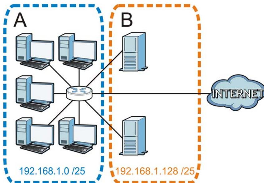
In a 25-bit subnet the host ID has 7 bits, so each sub-network has a maximum of  $2^7 - 2$  or 126 possible hosts (a host ID of all zeroes is the subnet's address itself, all ones is the subnet's broadcast address).
