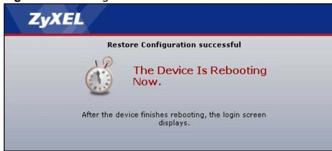
The NBG-418N v2 automatically restarts in this time causing a temporary network disconnect. In some operating systems, you may see the following icon on your desktop.
