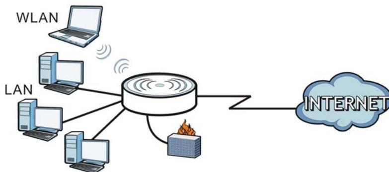
The LAN screens can help you configure a LAN DHCP server and manage IP addresses.
